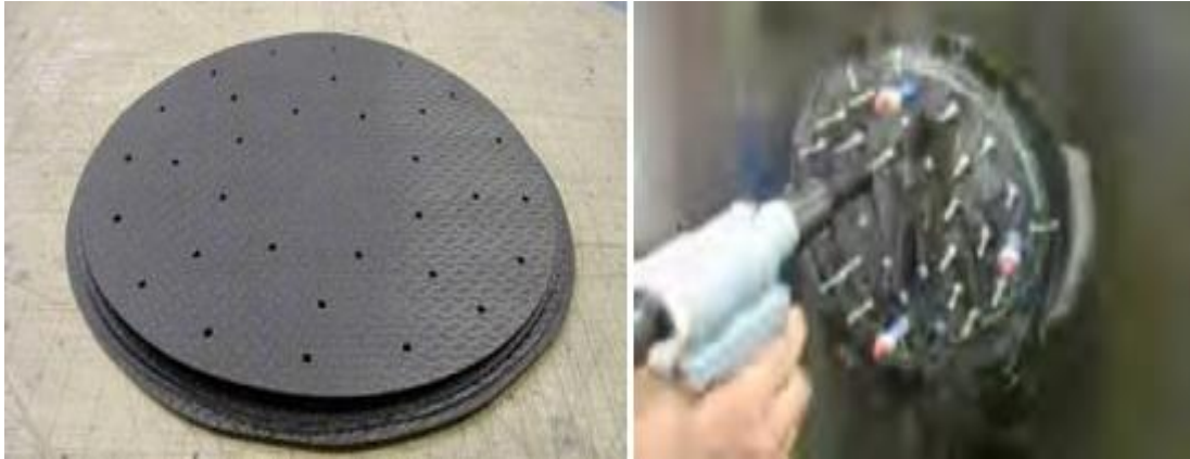
Figure III.14: Solution hybride de patch riveté/collé d'Eurocopter [31]
