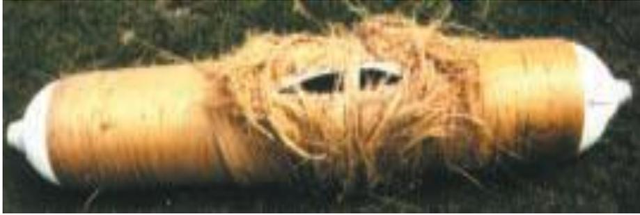
**Figure I-6 :** Réservoir GNV (type 2)
