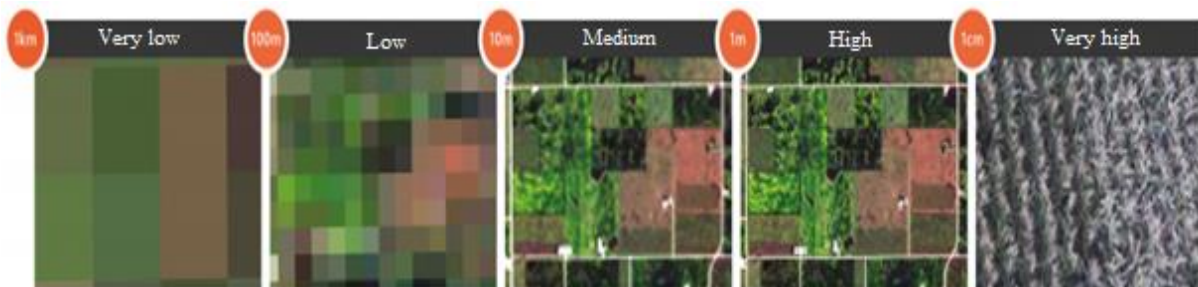
Figure GI.1. A scene with different spatial resolutions: from left to right 1Km, 100m, 10m, 1m and 1cm 1 .
