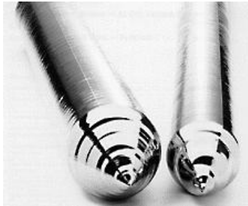
Figure III.5: Lingots de silicium monocristallin [12].
