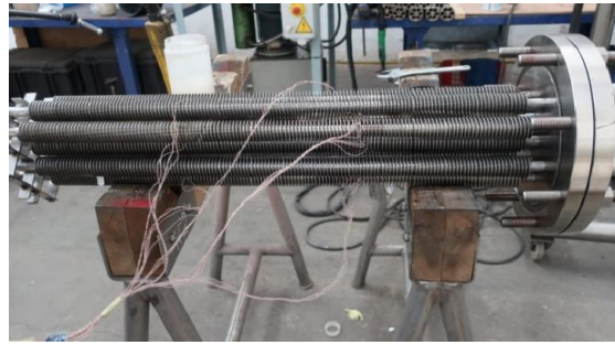
Figure 1.3: Latent thermal energy storage accumulator equipped by annular-finned tubes (ACCUSOL project).
