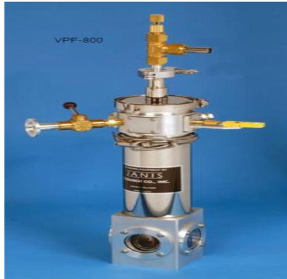
Figure II.3: Cryostat Janis VPF -800.
