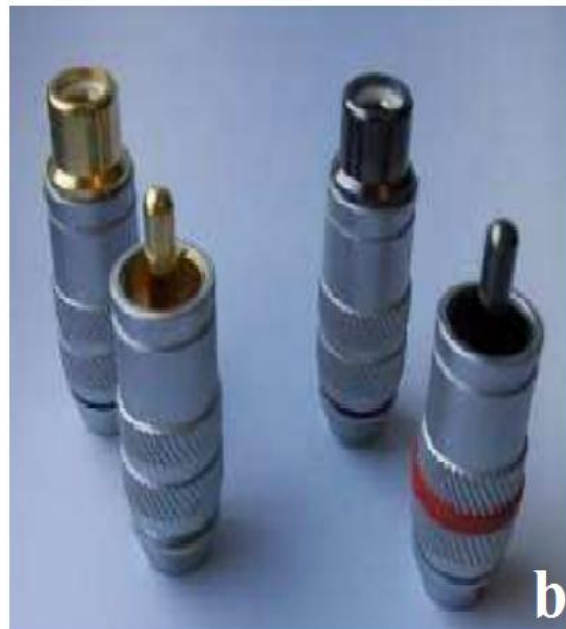
Fig I.8. (a): The Ti_2AlC is used as heating elements ( \sim 1400^\circ C ), (b): The replacement of the gold layer by Ti_3SiC_2 in the form of thin layers is carried out for electrical contacts coating [5,24].
