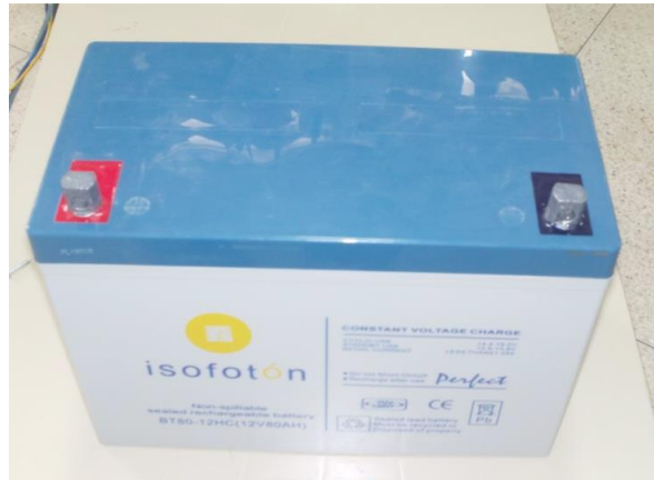
Figure III. 4. Batteries Isofoton 12V 80Ah
