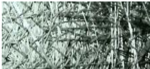
Figure I.10 : Fibres multidirectionnelles [Gornet, 2008]
