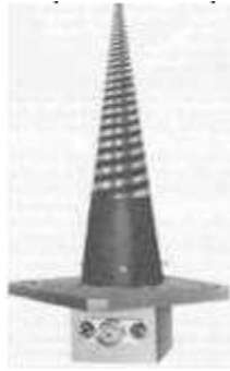
Figure II.6: Antenne spirale conique.
