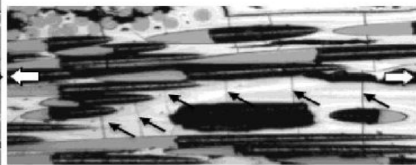
(c) Fissure intrafil
