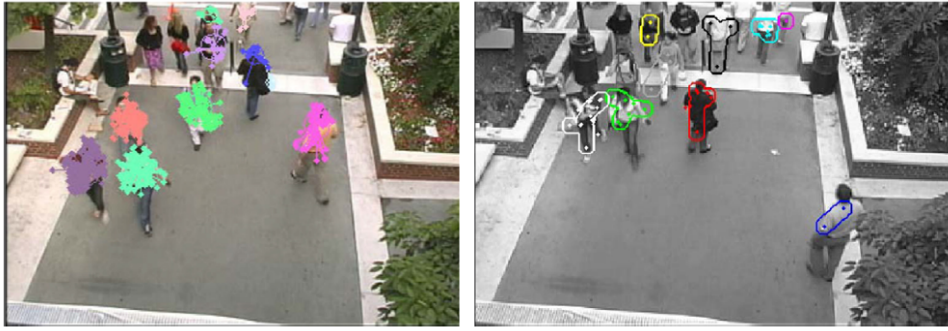
FIGURE 2.7: Trajectory clustering for people counting with results output from [12] on the left, and results output from [71] on the right.
