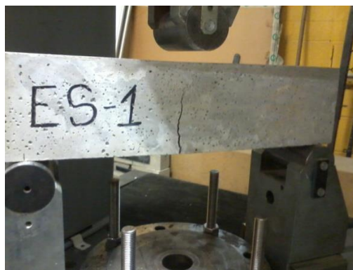
Figure 4-11 : Essai flexion trois points.
