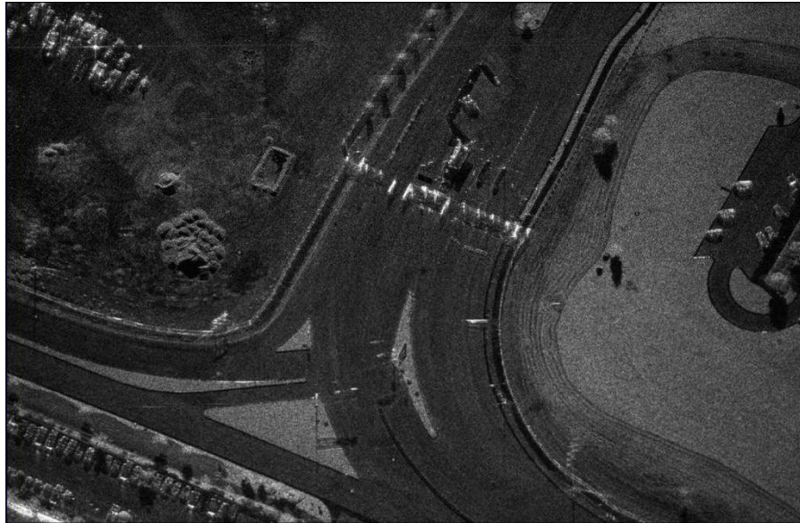
Figure 1.8 miniSAR 4-inch resolution K_u Band image, Kirtland Air Force Base Gated Entrance 9
