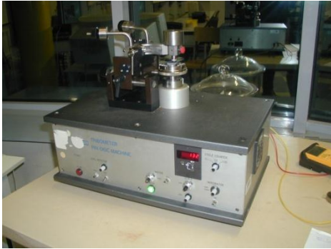
Fig. 2 Pin-on-Disk (PoD) tribometer from CSM instruments
