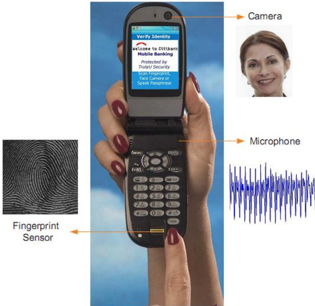
Figure 17. Mobile banking application [73].
