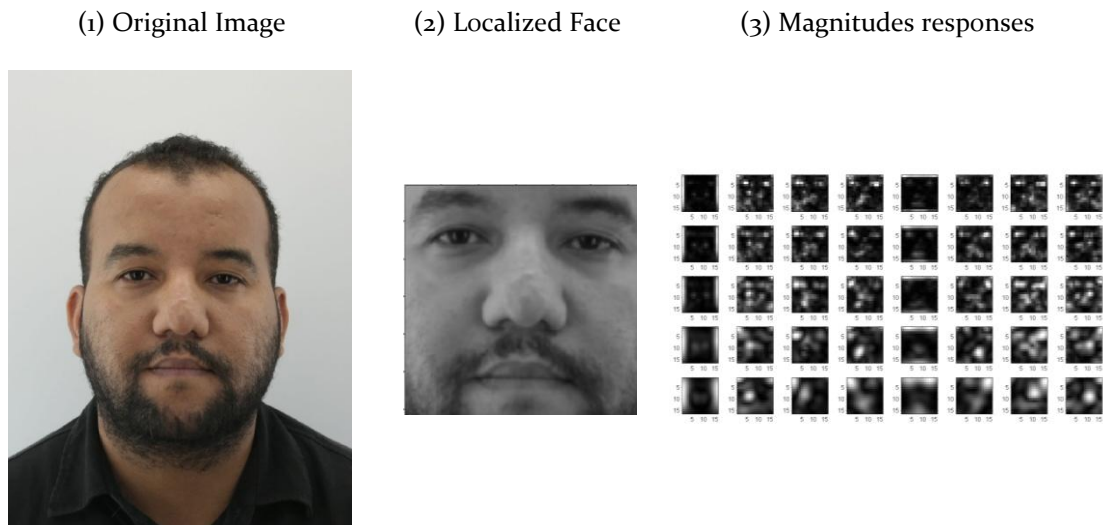
Figure 13. Magnitude responses of the filtering operation with the Gabor filter bank (no down-sampling) using the 24 th subject face in BIO database.
