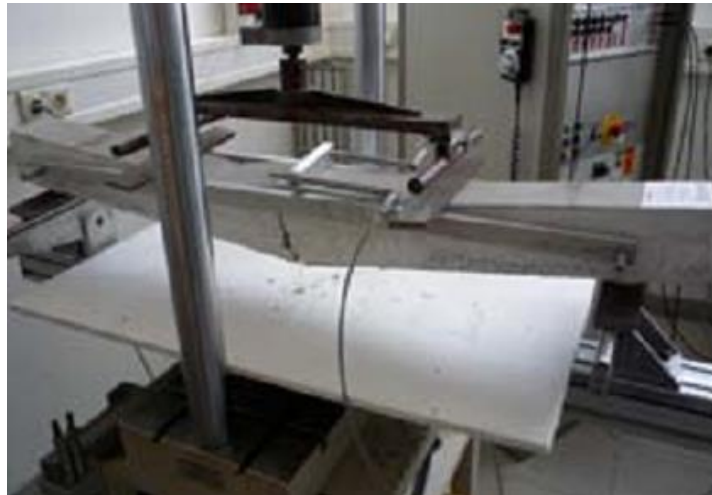
Figure II.2: Essai de flexion à quatre points, source: ILEK
